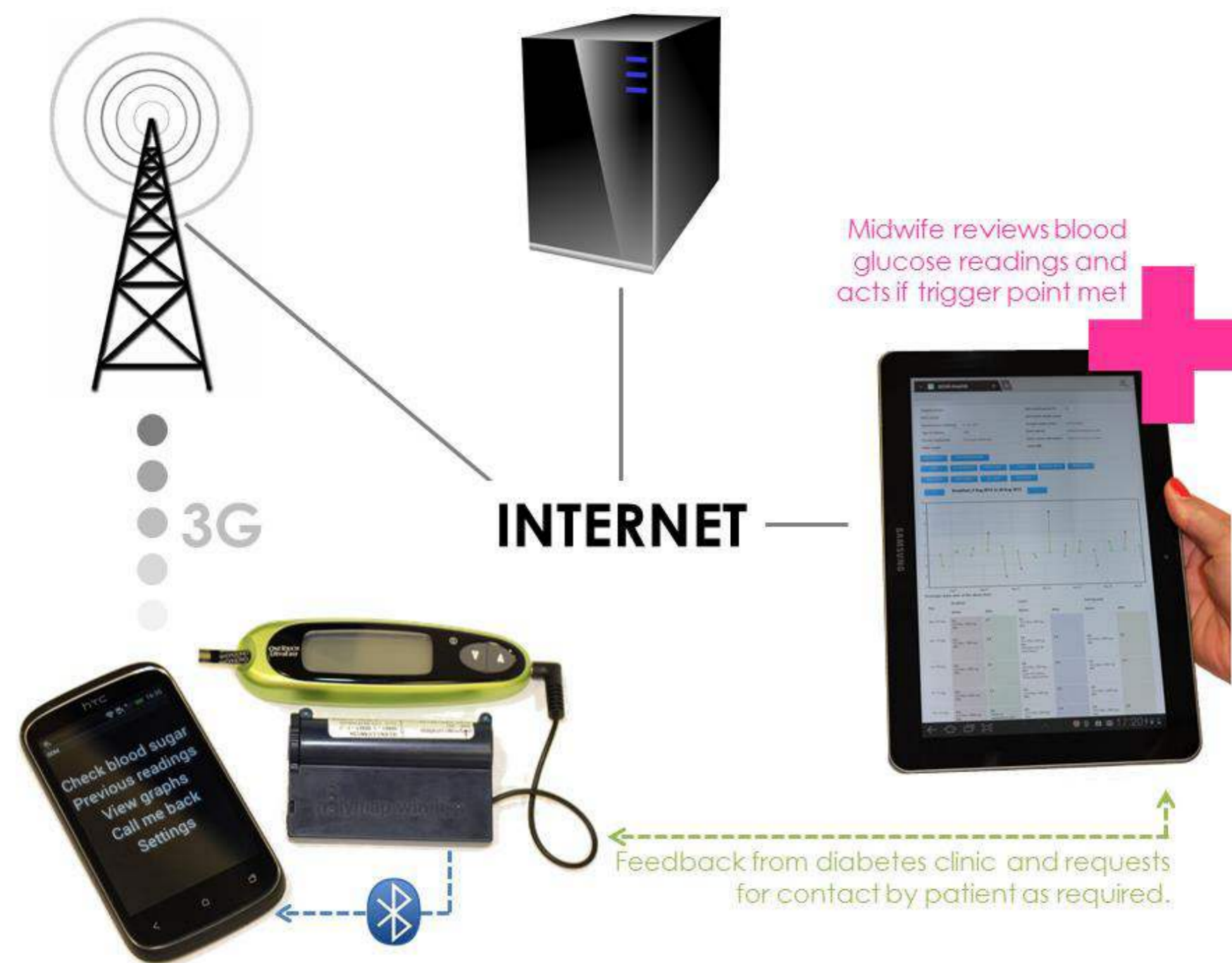
Figure 1: The GDM-Health remote blood glucose monitoring system
