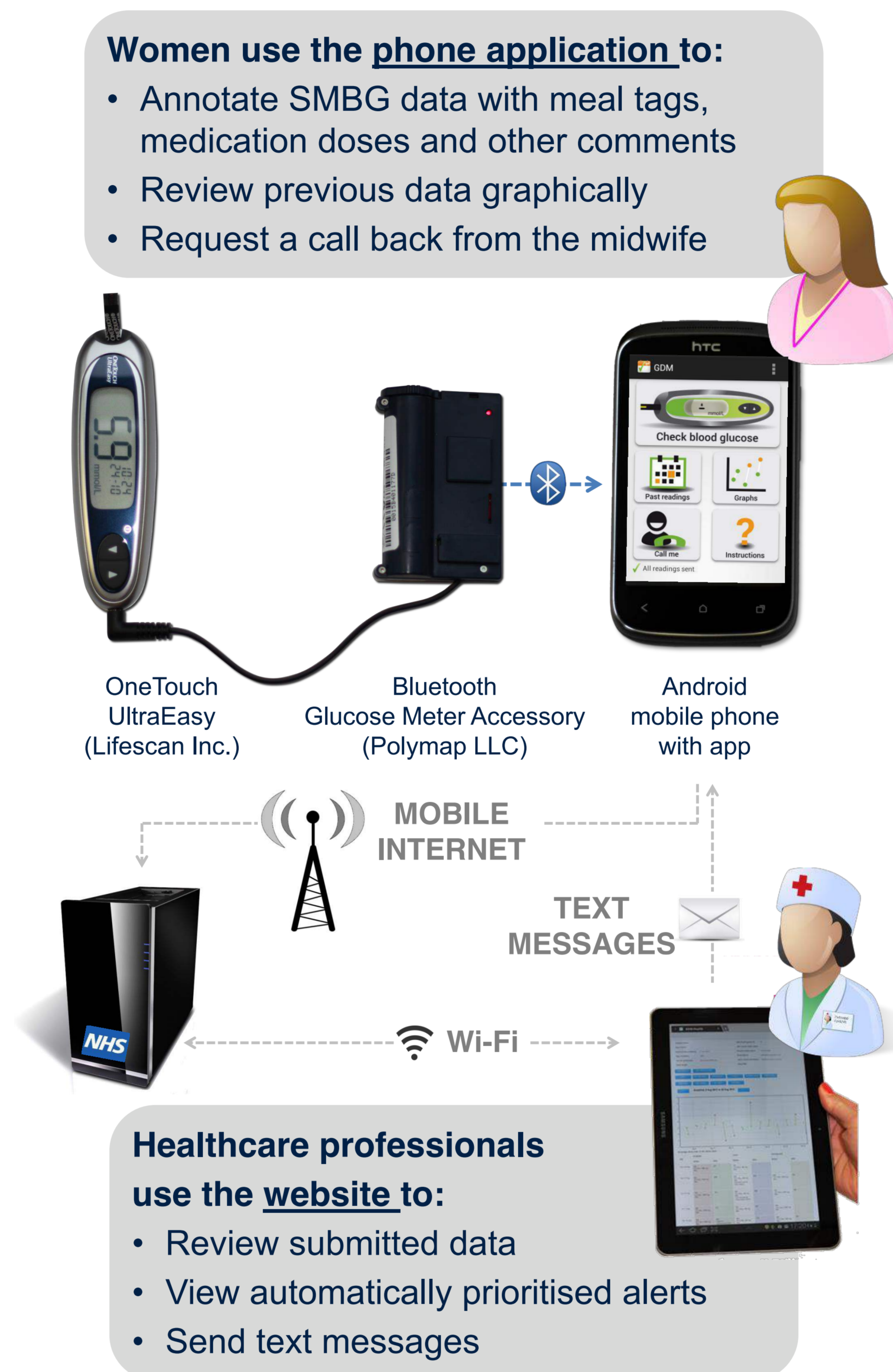
Fig. 1: Schematic of the GDM-Health system
